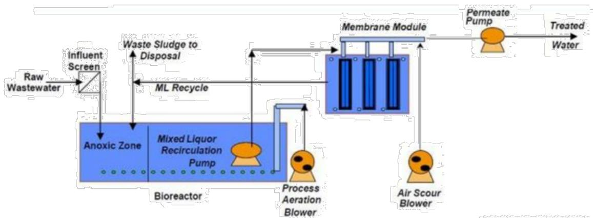
Figure 21 – Schematic diagram of MBR
