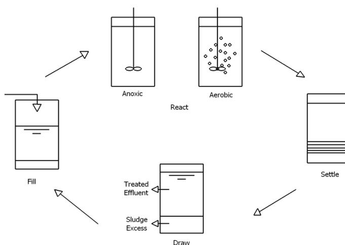
Figure 20 – Schematic diagram of SBR
