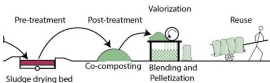
Figure 54 – Schematic diagram of Co-composting
