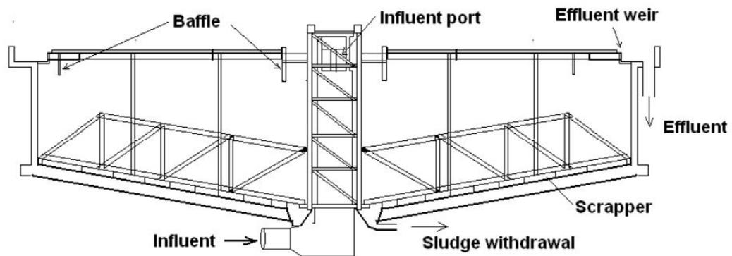
Figure 13 - Schematic diagram of primary clarifier
