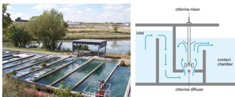
Figure 24 – Chlorination Basin (left), Chlorine dosing and mixer (right)
