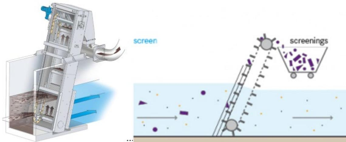
Figure 11 - Schematic diagram of screens
