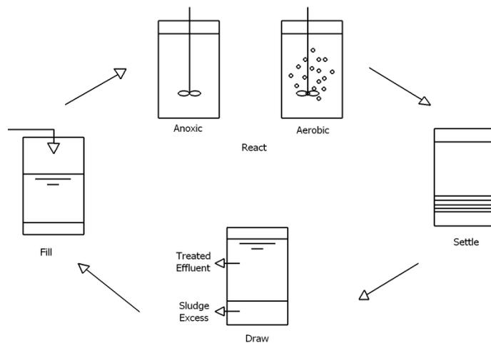
Figure 20 – Schematic diagram of SBR
