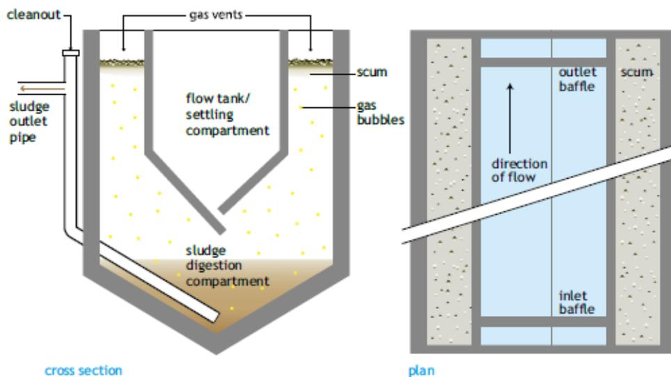
Figure 44 – Schematic diagram of Imhoff Tank
