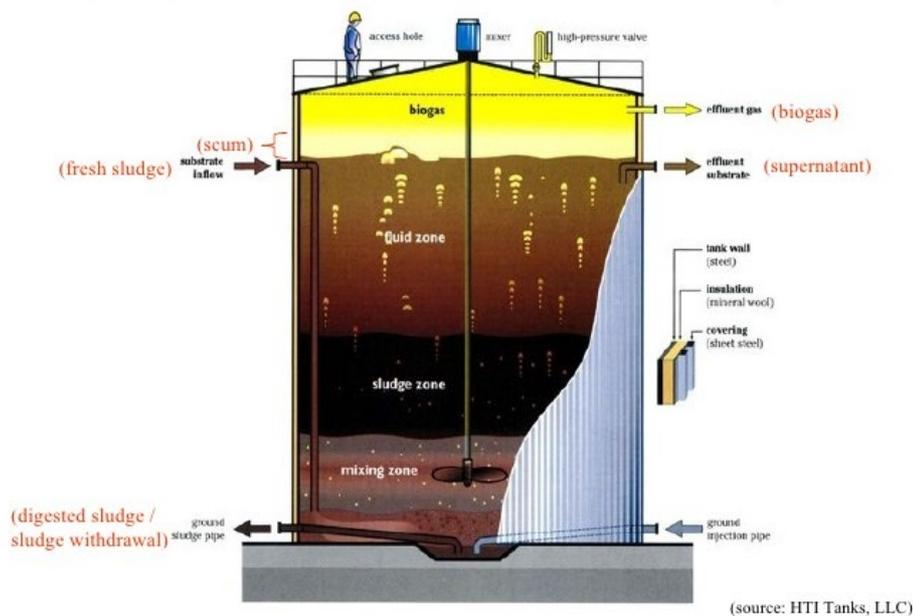
Figure 43 – Schematic diagram of Anaerobic Digester
