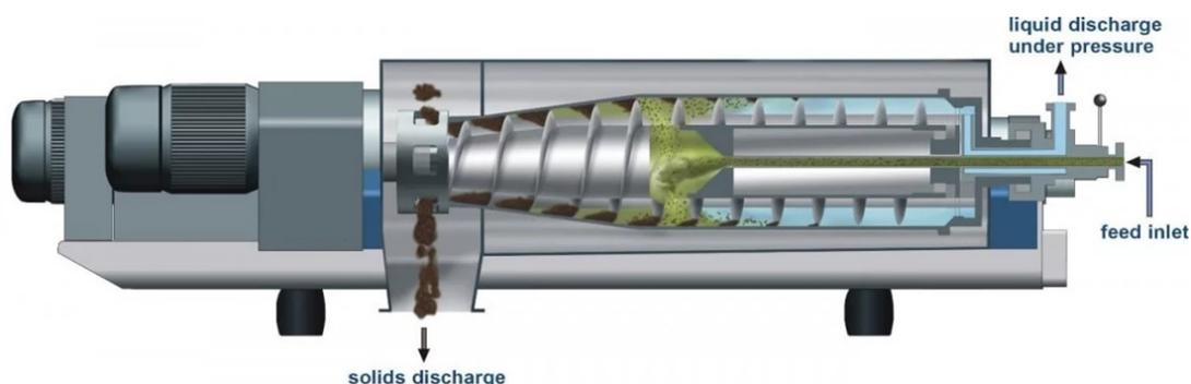
Figure 48 – Schematic diagram of Centrifuge
