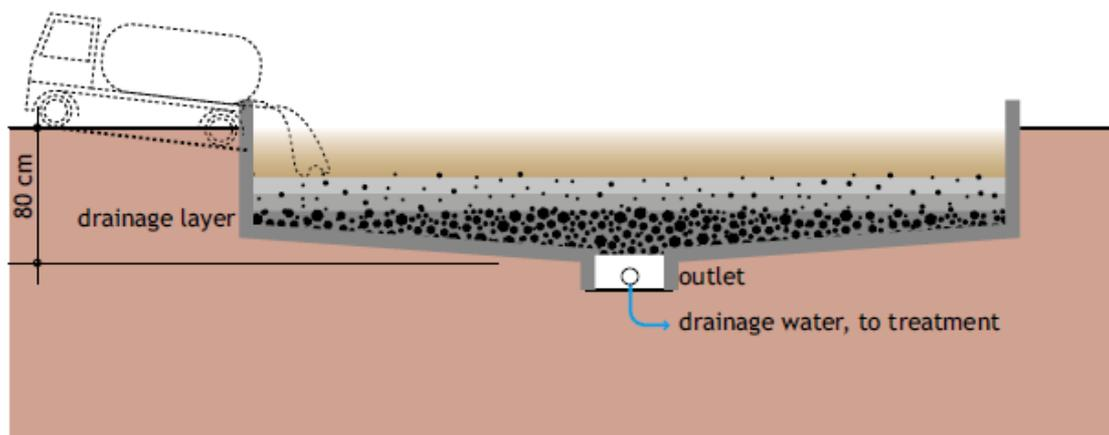
Figure 46 – Schematic diagram of Unplanted Drying Beds
