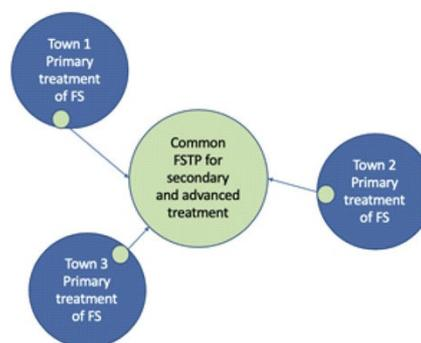
Figure 56 – Planetary Model
