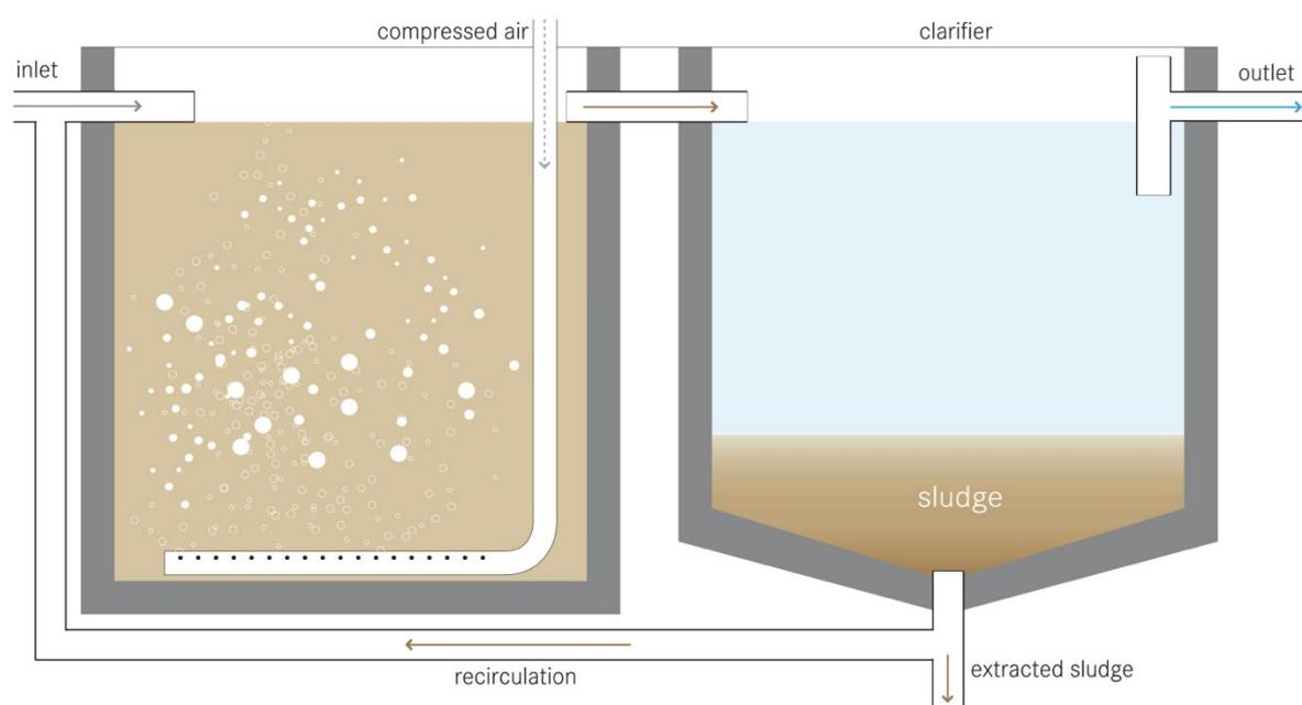
Figure 19 – Schematic diagram of ASP
