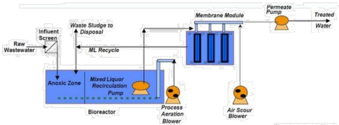
Figure 21 – Schematic diagram of MBR
