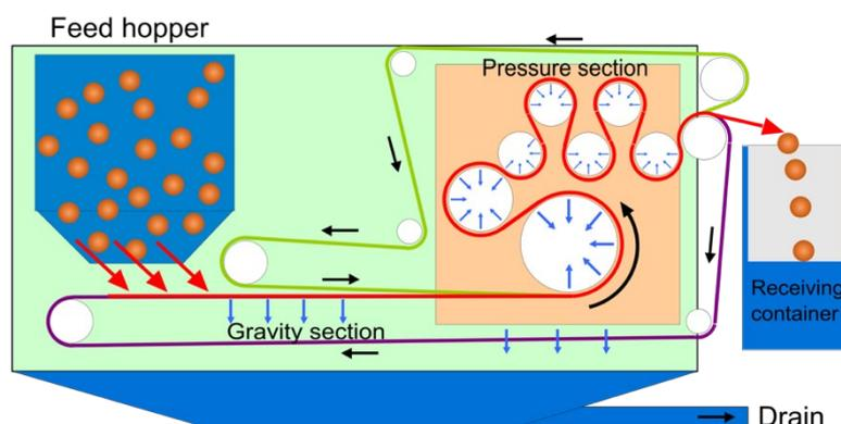
Figure 50 – Schematic diagram of Belt Press
