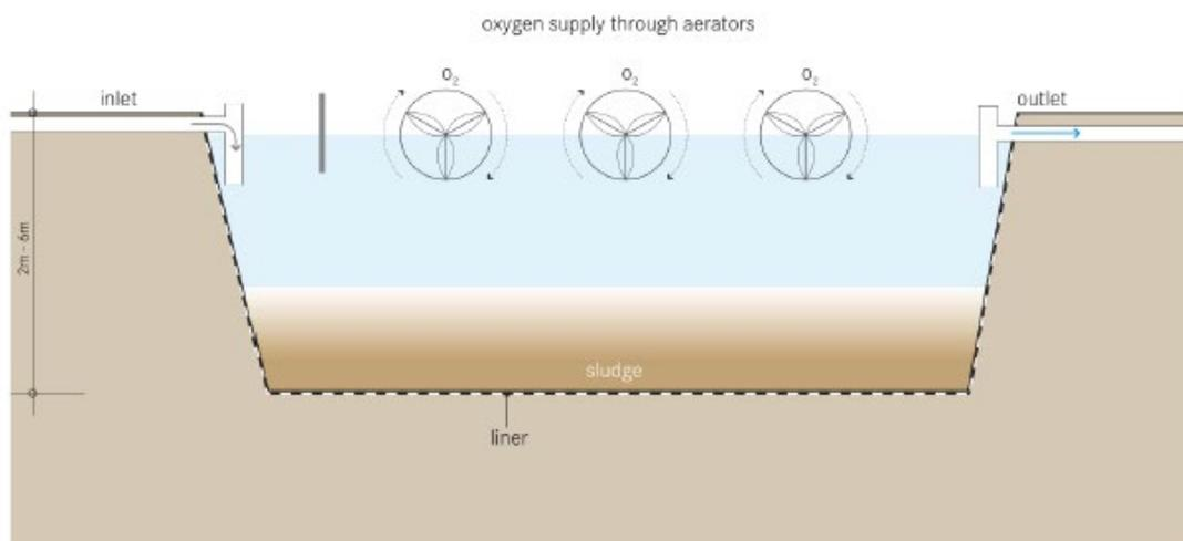
Figure 23 – Schematic diagram of aerated pond
