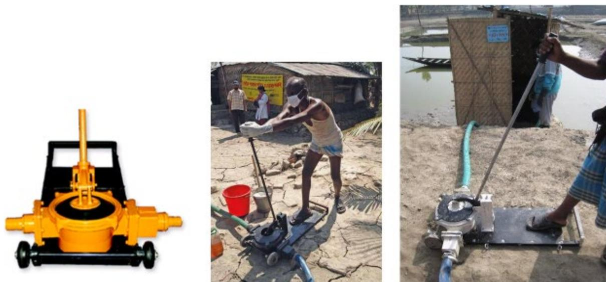
Figure 36 – Manually operated Diaphragm pump
