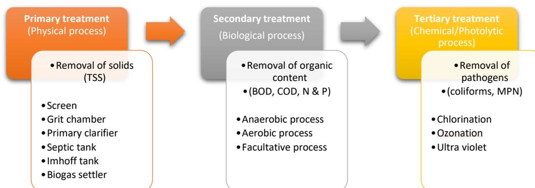
Figure 10 – Wastewater Treatment Chain
