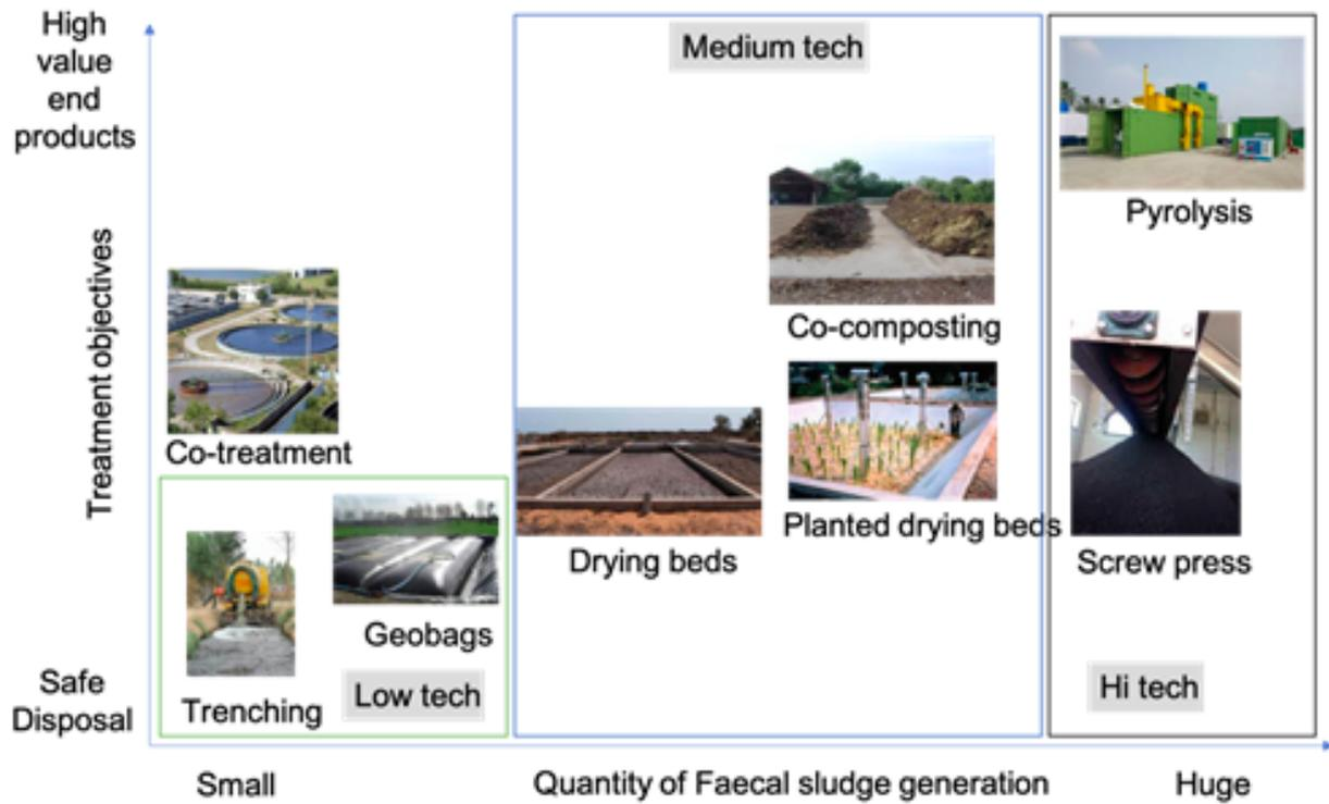
Figure 58 – Selection of treatment approach for Faecal Sludge/Septage
