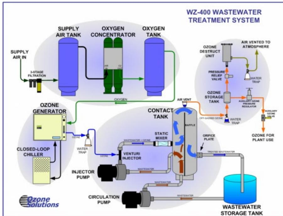
Figure 25 – Schematic diagram of Ozonation
