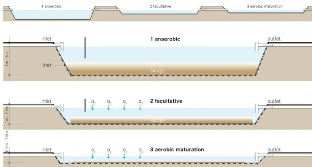
Figure 17 – Schematic diagram of WSP
