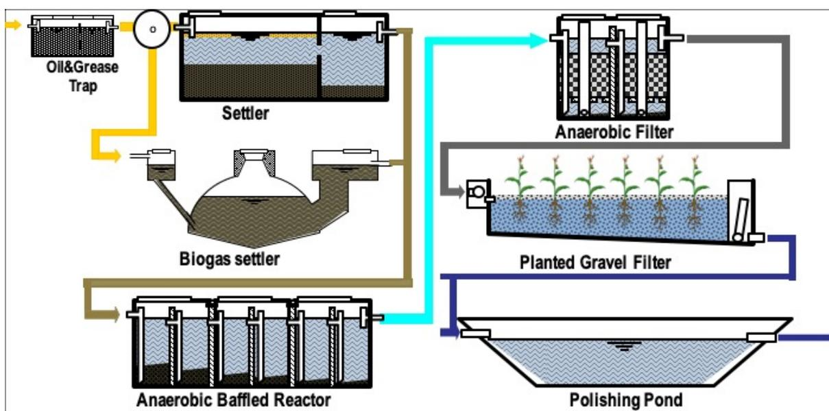
Figure 26 – Schematic diagram of DEWATS modules
