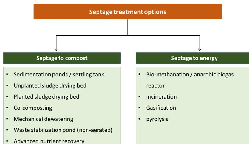
Figure 64 – Faecal Sludge/Septage Treatment Options
