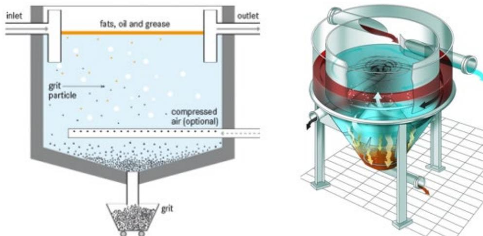
Figure 12 – Schematic diagram of grit chamber
