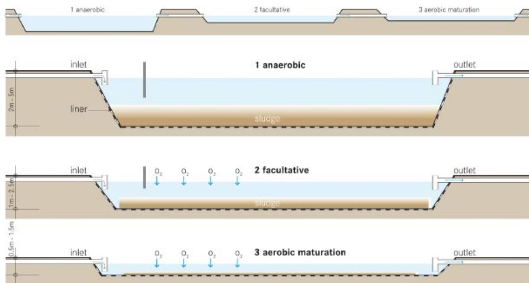
Figure 17 – Schematic diagram of WSP
