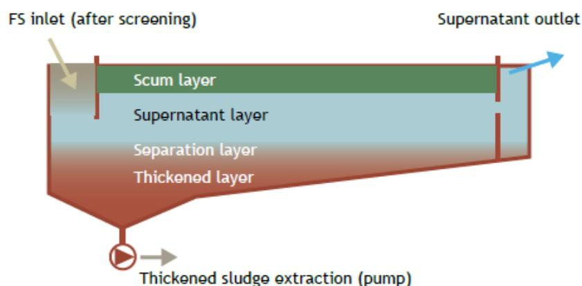
Figure 45 – Representative diagram of Settling – Thickening Tank
