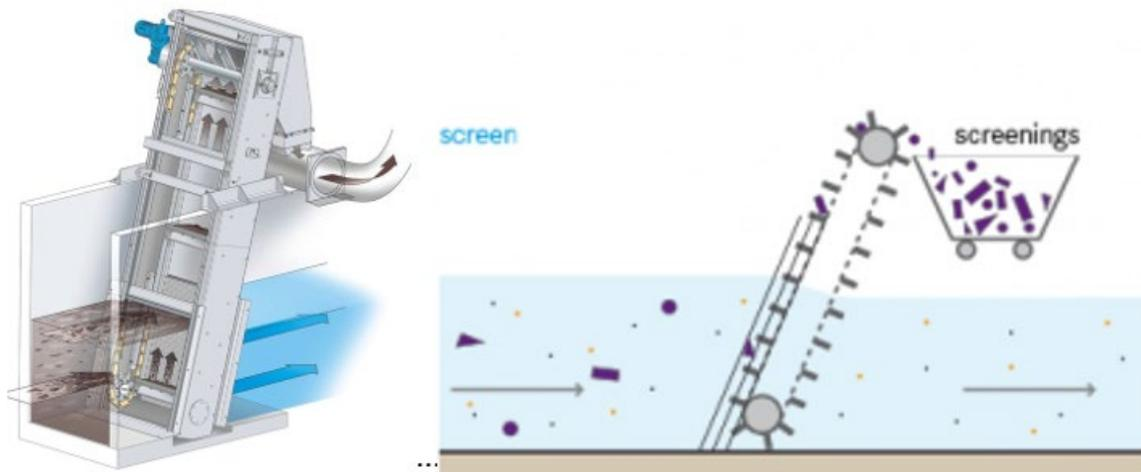
Figure 11 - Schematic diagram of screens
