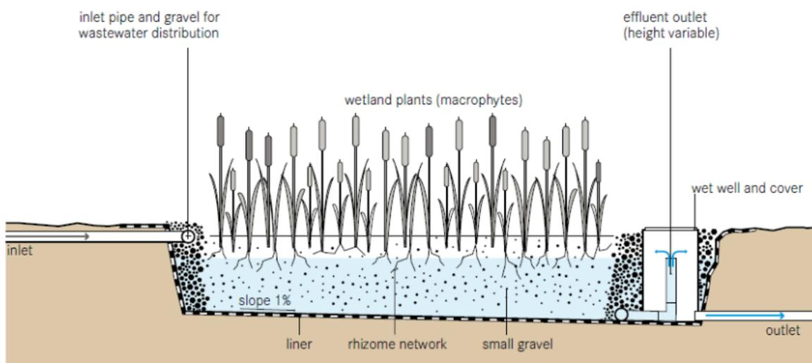
Figure 22 – Schematic diagram of horizontal flow constructed wetlands
