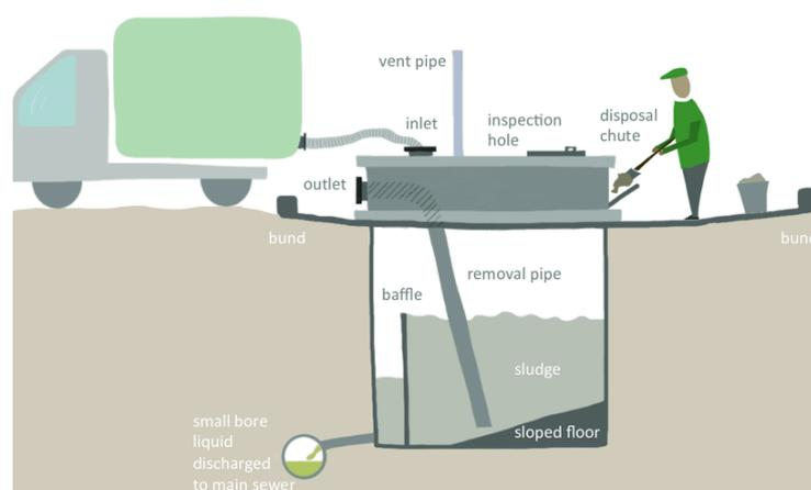
Figure 39 – Fixed type transfer station
