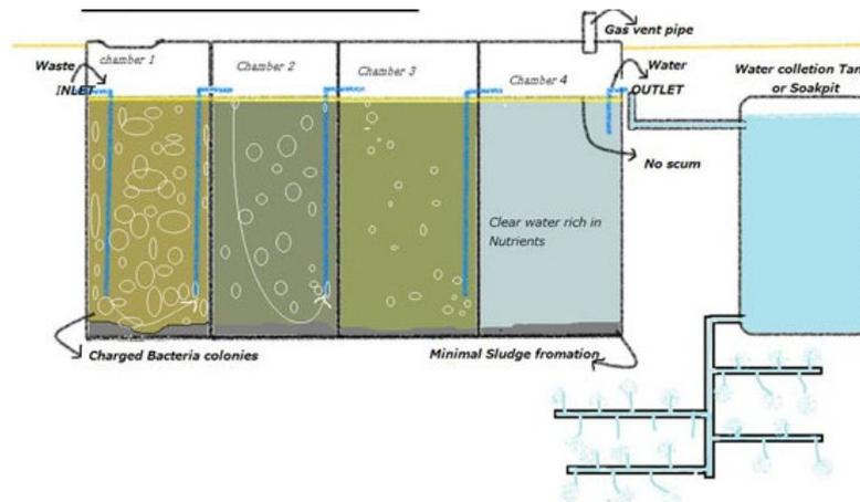
Figure 32 – Bio-digester tank system
