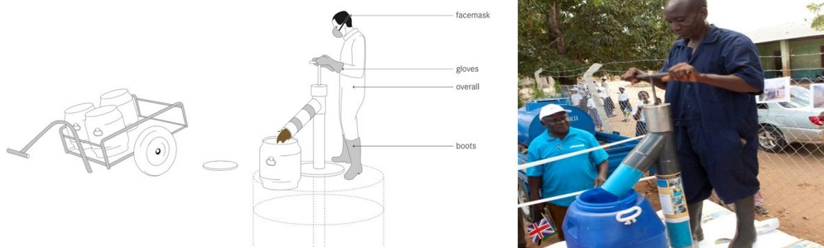
Figure 35 – Human powered emptying of OSS- Gulper
