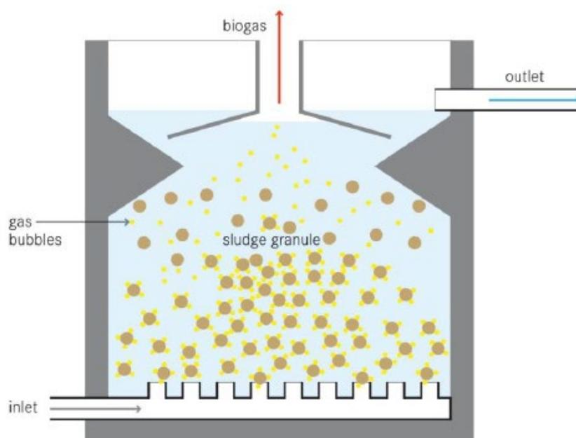
Figure 18 – Schematic diagram of UASB
