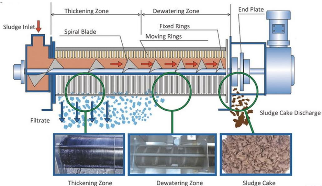
Figure 49 – Schematic diagram of of Screw Press
