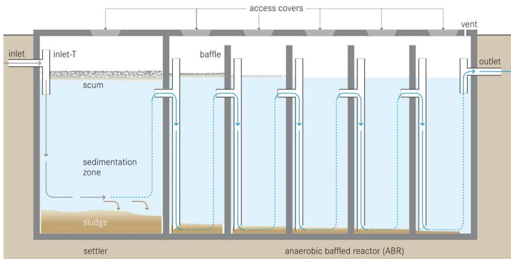
Figure 33 – Schematic diagram of ABR
