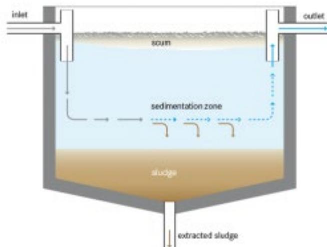
Figure 16 – Schematic diagram of Anaerobic/biogas Settler
