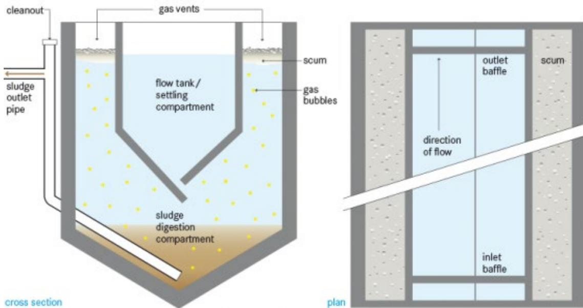
Figure 15 - Schematic diagram of Imhoff tank
