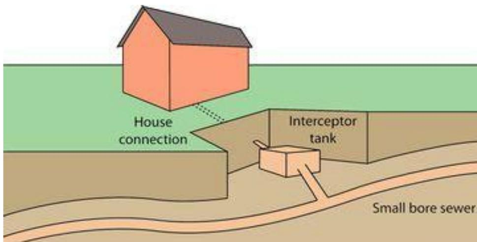
Figure 8 – Schematic diagram of small bore sewer system
