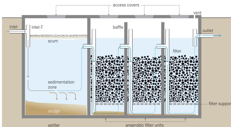
Figure 34 – Schematic diagram of Anaerobic Up-flow Filter
