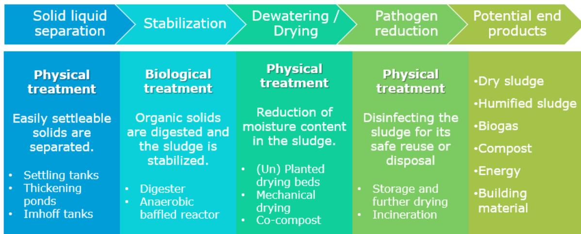
Figure 41 – Faecal Sludge and Septage Treatment Chain
