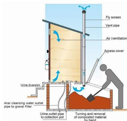
Figure 31 – Urine diversion and composting toilet (Ecosan)
