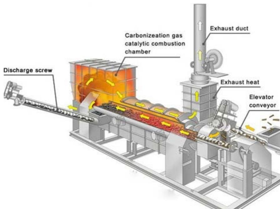
*Figure 51 – Schematic diagram of Sludge Incineration Plant*
